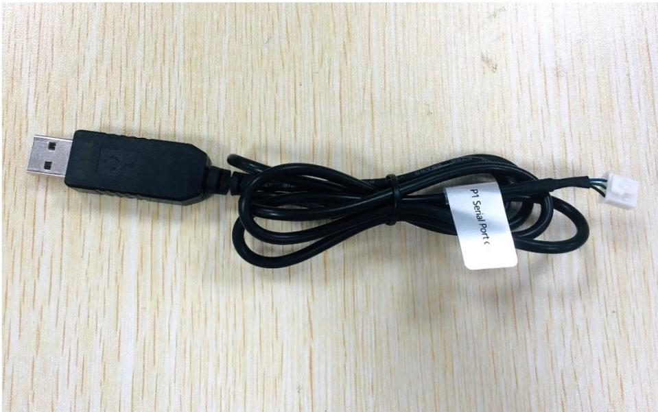
Loosen the 6 fixing screws of the top cover of the fixed marking machine (please keep the screws), move the top cover to the right, move it to see the auto focus plate, and connect the USB cable to the auto focus plate “UStart” interface, the other end is connected to the computer end.
