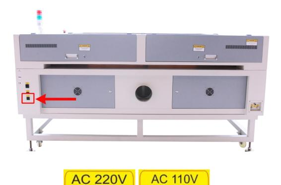
Tips: Do not connect the air compressor or the water chiller to the above interface, if connect them to the above interfaces that cause in failure of the machine, the warranty does not covered.
