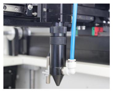
4" laser head owns a longer focal distance than 2" standard head, thus for cutting thick material, it makes the cutting edge more smooth and straight.
