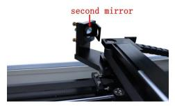
Make sure the power of the laser machine is turned off while cleaning. The 2<sup>nd</sup> mirror is installed on the left side of X rail. For the second mirror, you can clean them directly.
