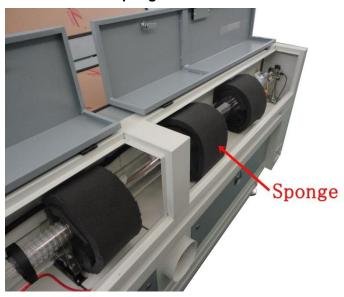
2. Take out the nylon cable ties around the honey comb plate and X axis. Remove the transparent bag out of the first mirror mounts, the second mirror mounts, the first mirror mounts and the standard laser head. Then install the laser head. Like below:
