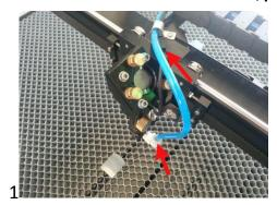
Remove the air pipe and the autofocus
