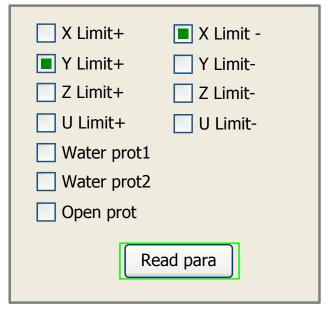
This interface shows some system input information, such as limiter status, the status of the water protecting, and the status of the foot switch etc.. When the input is validated, the color frame will be green, otherwise it's gray.
