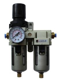
When we use the High pressure air compressor for blowing air, it will absorb much moisture with air at the same time. If we just let the moisture go, they will gather on the focus lens, and when the laser working, the water (moisture) will heat that may lead the lens break. Thus we need a water separator for help, it can stop moisture reaching lens. Water separator was installed between the air compressor and laser head.
