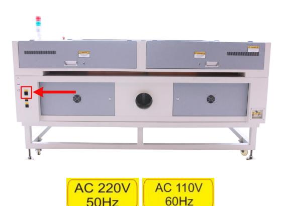
Tips: The main fuses are located inside the connection socket and are accessible from the exterior.
