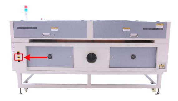
The input voltage must correspond (AC 220 V/50 Hz or AC 110 V/60 Hz) – see information label beside the connection socket.
