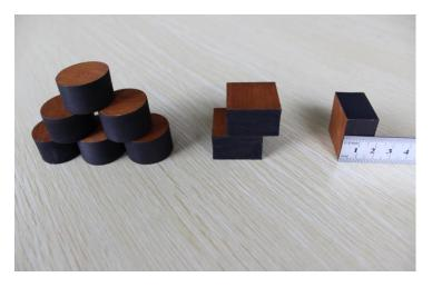
Note: when we cut thick material (usually more than 10mm) with 4" laser head and the material are very easy to catch fire, for example: wood, foam, plastic, etc. usually we would suggest customer to use a High pressure air compressor set while working.
