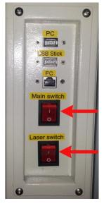
If all covers are closed, immediately after being switched on, the device starts the referencing process. When the referencing process is completed correctly, an acoustic signal sounds and the device is ready for operation. The operation panel will display the home screen when the laser is completed resets.
