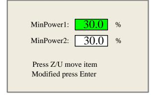
When "Z/U" key is pushed, the green block can move up and down to denote the changing item, then "Y+/-" keys and "X+/-" keys can be used to change the value.
