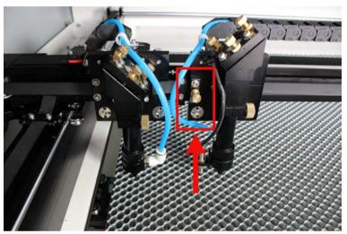
2. It's the x-axis working length is 1600mm, but we added a laser head to here. So we have to set the x-axis working area to 1500mm even smaller.
