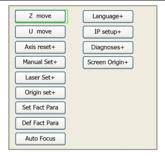
Press up and down arrow keys to move the green block to the anticipant item, and then push the "Enter" key to display the sub menu.
