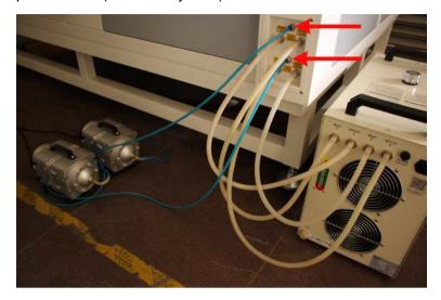
The input voltage must correspond (AC 230 V 50/60 Hz or AC 115 V 50/60 Hz) – see information label beside the connection socket.
