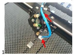
Remove the air pipe and the autofocus
