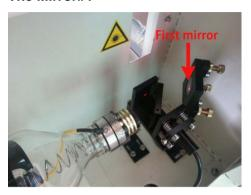
The mirrors are easily get dirty. And this will reduce the efficiency of the laser beam. Meanwhile, laser energy absorbed by the mirror may cause heat and destroy the mirrors too. For the first mirror, you can clean them directly.
