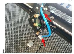
Remove the air pipe and the autofocus
