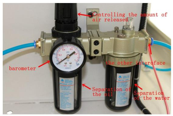
5. After the devices are all connected properly; please turn on the switch of the air compressor, then the air compressor will exhausting and blowing air, and the air will go through the oil-water separator for separating oil and water, and then the air will flowing to the laser head, here the laser will working properly. See as below:
