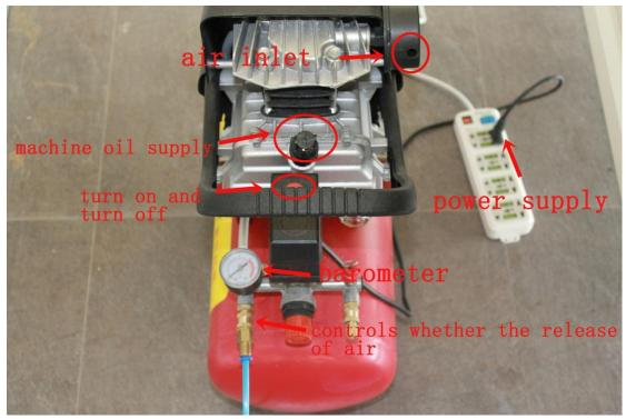
4. Introduction of the oil-water separator, this part controls the air releasing or not and the amount of the released air, it can be adjusted by the black switch; and there are two containers for separating oil and water. Generally speaking, "the other interface" of the oil-water separator has been connected before out of factory. Users needn't to connect this interface. See as below:
