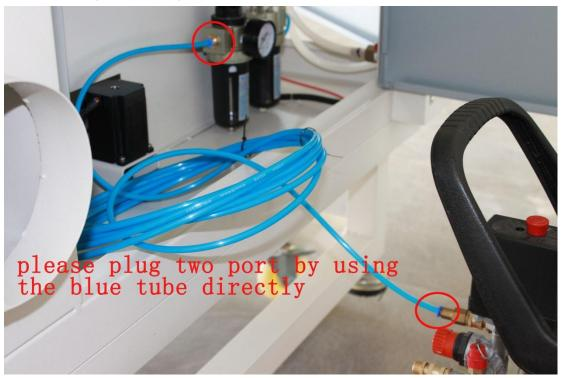
2. Unplug the interface of the white pipe that connected with the air pump, and connect the white pipe with the blue pipe (this blue pipe has been connected with and fixed inside the machine). See as below:
